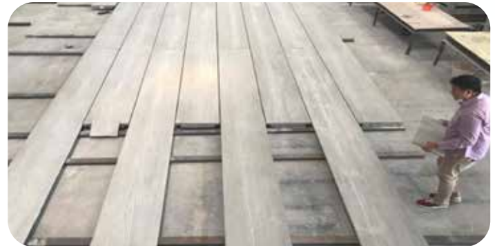
B. Timber Texture Board Form Glass Fiber Reinforced Concrete (GFRC) Panels: Inspection and mock-ups are essential to establish the buildability and quality of the Timber Texture Board Form GFRC Panels
