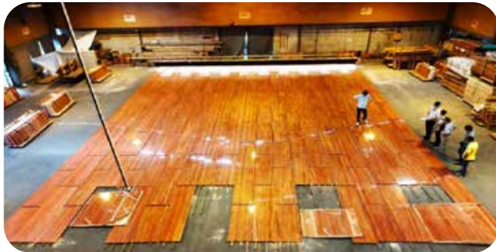
A. Red Travertine Dry Lay: A dry lay was added to the red travertine to ensure quality turnout in meeting the required colour, tonality and vein match.
